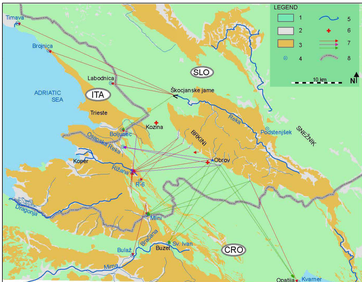
Figure 3.03: Hydrogeological map of the area between Trieste and Kvarner bays of the Adriatic sea with underground water connections (from Petrič et al. 2007). Legend: 1. Karst-fissured aquifer, 2. Porous aquifer, 3. Very low permeable rocks, 4. Karst spring, 5. Surface stream, 6. Location of oil spillage, 7. Main, secondary and uncertain underground water connection, 8. State border.
